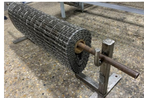
New belt in staging area on jack stands.
